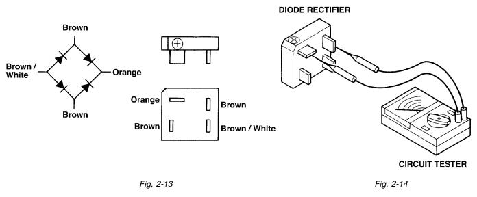
Circuit inside of the diode rectifiers is as shown in Fig. 2-13. Check continuity between each terminal by using a circuit tester as shown in Fig. 2-14. The rectifier is normal when condtinuity is as follows:
